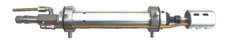
PIPECOATER-III/125 tool is designed to coat the inside of pipe or tubing ranging from 76 to 125 mm (3" - 5") ID without the need to rotate pipe or tubing and to apply an even paint film thickness throughout. Generally, any type of coating may be used in this tool that can be airless sprayed.
