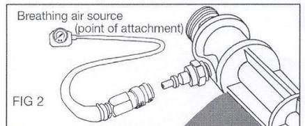
**!WARNING!** Make sure you understand the breathing air pressure table before using the respirator. Make sure you set the correct air pressure for the correct supply hose length.
