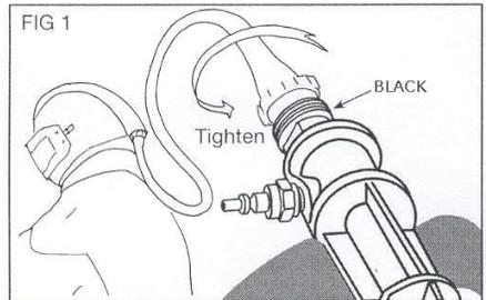
3. With air flowing through the respirator, adjust the air pressure at the point of attachment to the recommended air pressure specified in the COLD AIR, BREATHING AIR PRESSURE TABLE.
