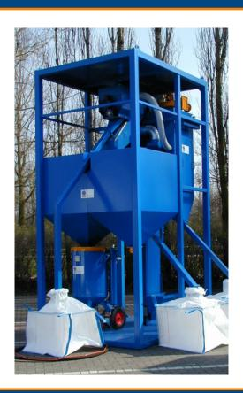
The RC-80-160 is an abrasive recycling system which can be used inside or outside. Several types of reusable abrasive can be recycled by the RC-80-160 **into bigbags or blast vessels**. The rate of recycling depends upon the type of abrasive being processed. Garnet can be recycled at a rate of up to 11 tons per hour, steel abrasive can be recycled at a rate of up to 21 tons per hour\*.
